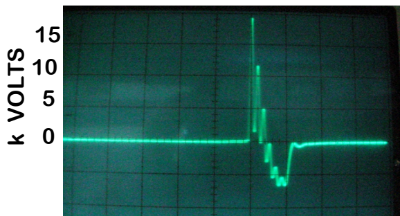
Figure 8 OSCILLOSCOPE OF SPARK PULSE (FILE PHOTO FOR REF. ONLY)
