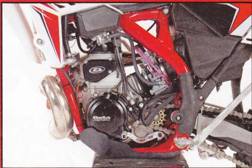
The motor might look somewhat familiar, but it's all new, with the electric-starter motor hidden under the gearbox.
