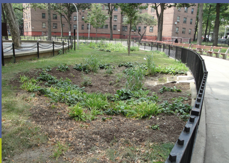
Fig. 5-5. Rain garden capturing sidewalk run-off in New York City (Image: Hazen & Sawyer)
