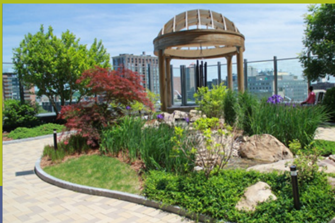
Fig. 5-9. A green roof garden at the Smilow Cancer Center at Yale-New Haven not only acts as an outdoor space and meditation garden for patients, but also absorbs, filters, and slows stormwater runoff from the roof. (Image: Save the Sound)
