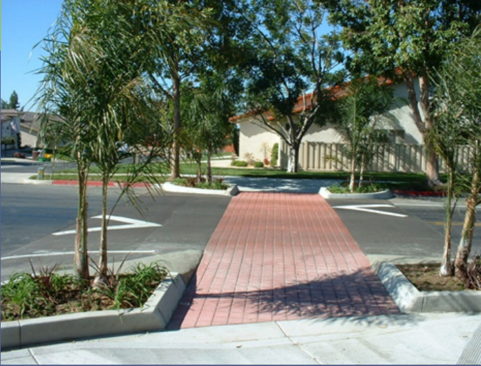
Fig. 3-3. A raised crosswalk in Oceanside, California. In this example, decorative materials have been used for the crosswalk to further increase visibility of pedestrians crossing. (Image: WalkSanDiego)
