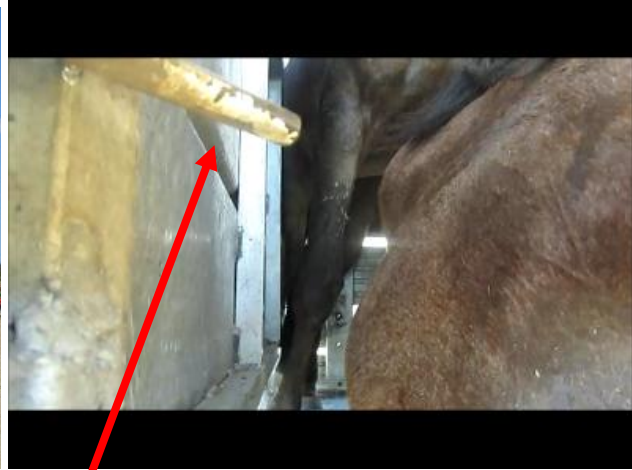
Broken piping inside trailer
