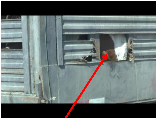
Hole in trailer side – horses' legs can get stuck
