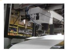
The MCT360 measures water based EMULSION COAT WEIGHT on the wet end. The strong Near Infrared signature of water and known liquid/solids ratio allow for very fast and very accurate measurements in real time. Accuracies are typically +/- 0.15 gsm.
