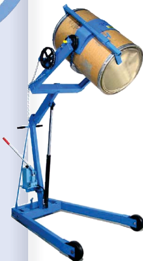
Model 400A-72 Capacity: 800 Lb. Pour height: 72" Hand pump drum lift Chain wheel drum tilt Shown with MORcinch™ Bracket Assembly Option # 4556-P (sold separately)
