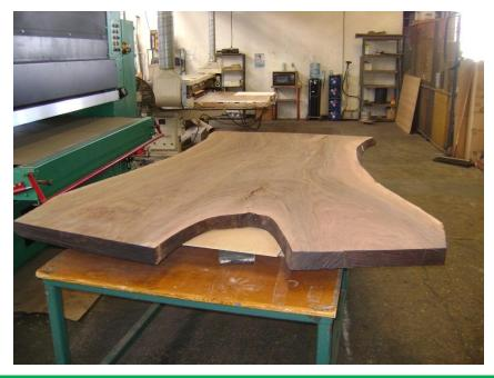
This Slab is 112" long & 80" across the ears of the crotch. It was sanded with 60x belt and came out nice and smooth with a +/- .005" thickness variance from side to side.
