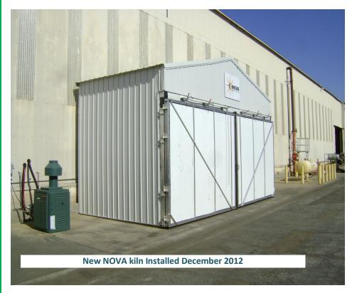
Our new high capacity kiln can any dry types of wood With products. programmable controller, the kiln can run an infinite number of drying "recipes". With expert planning and tracking of drying schedules, this kiln gives us the ability to produce a wide variety of stable products ready for incorporation into your designs.
